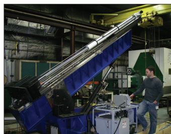
Convertible Test System 20,000 lb load - 100" CC
