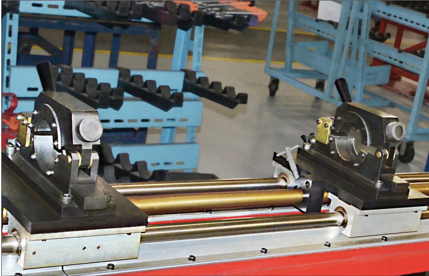
Nook/Thomson slide rail system used as a steady rest for a large diameter CNC machine.
