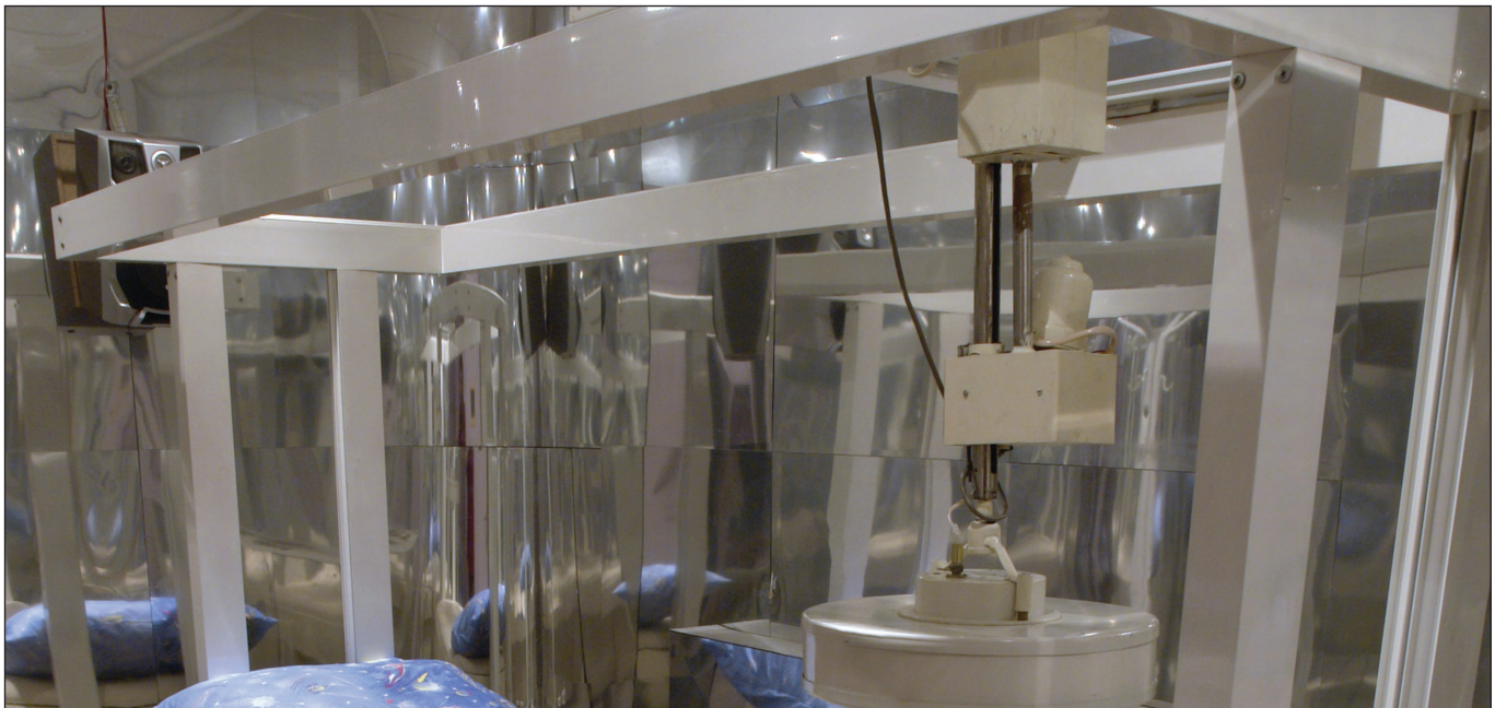
Nook/Thomson Linear Shafting and Bearings used to guide a loader for medical waste processing.
