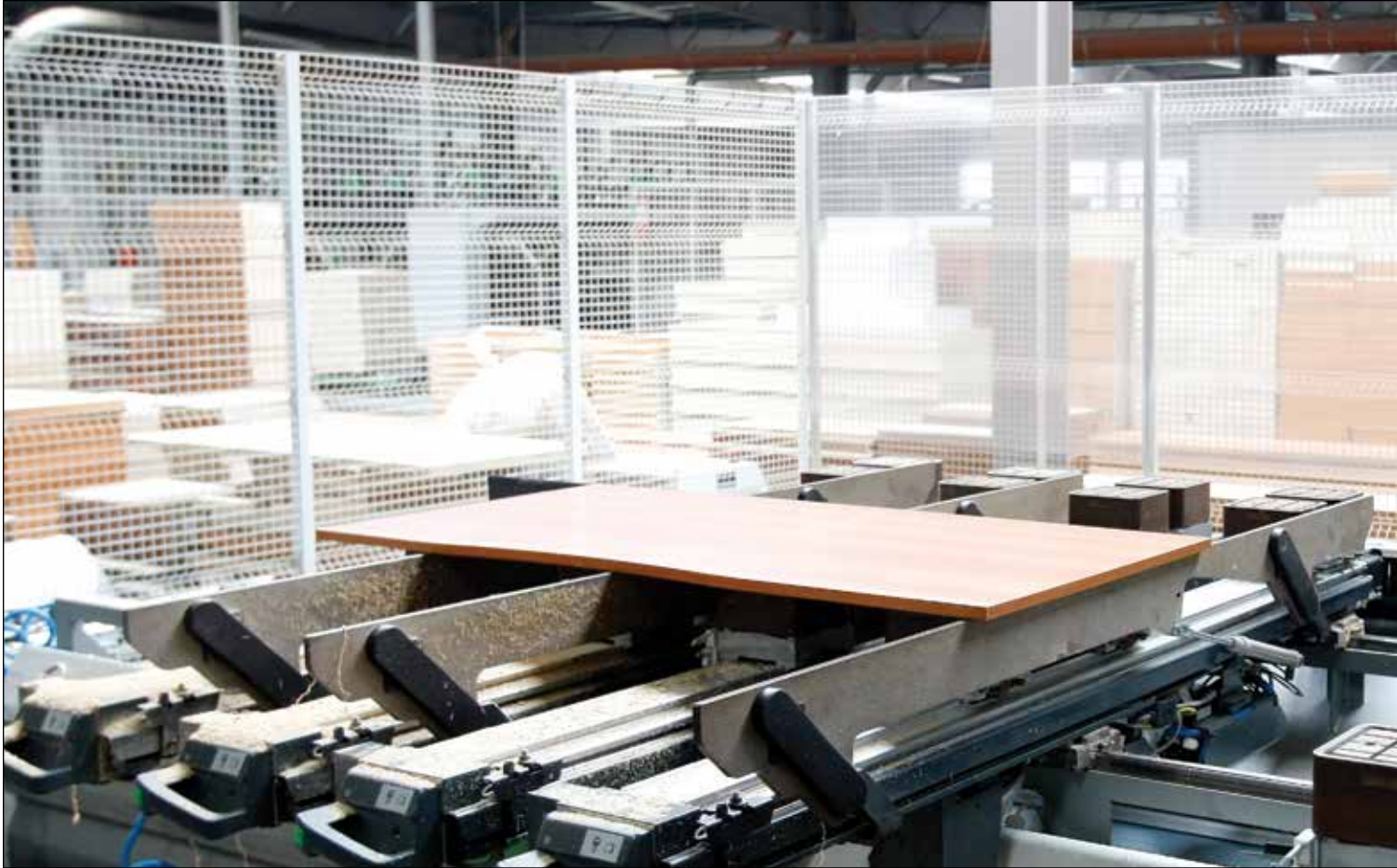
Nook/Thomson Modular Linear Actuators used in an automatized wood factory.
