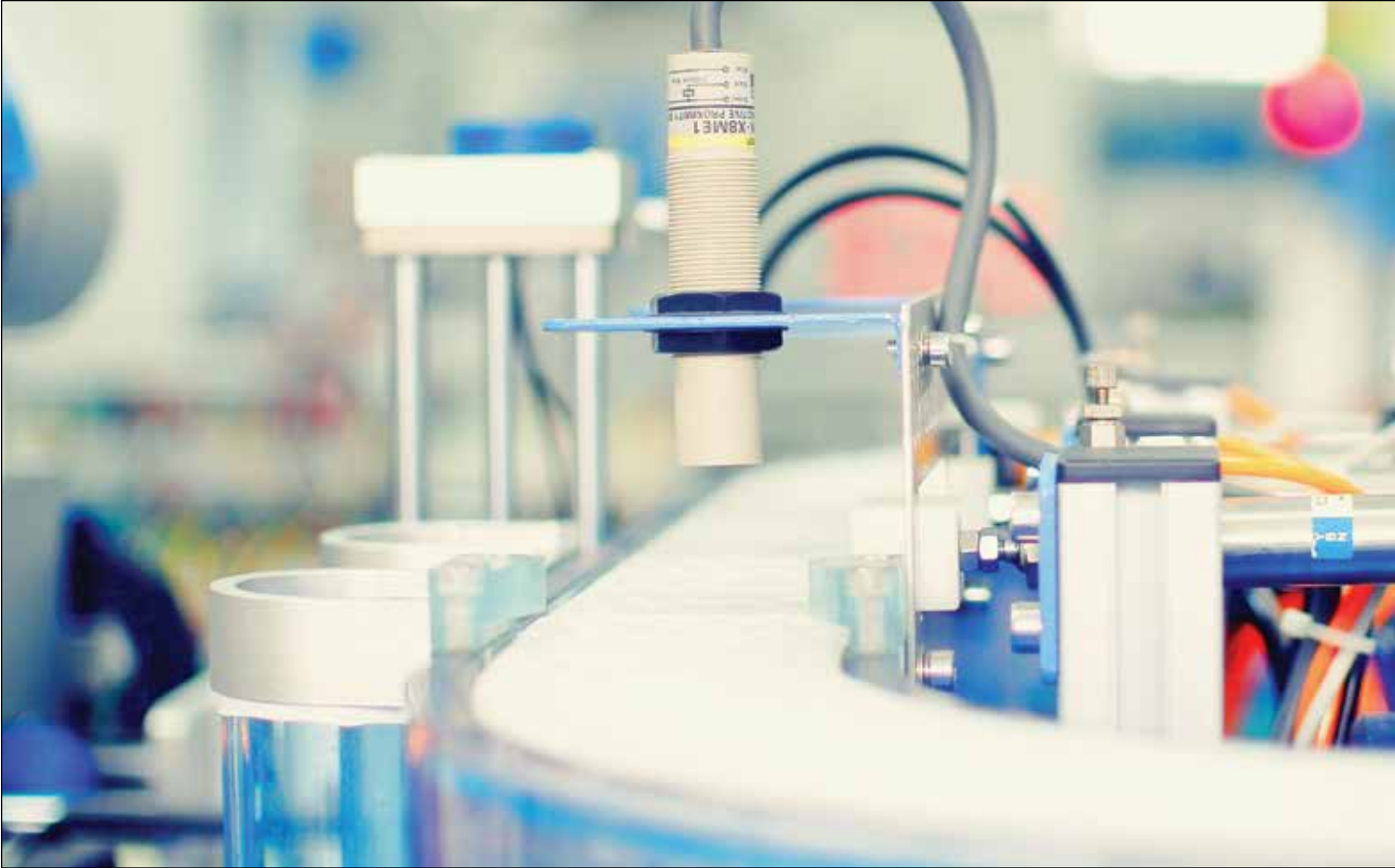
Nook/Thomson Modular Linear Actuators used in a medical automation application.
