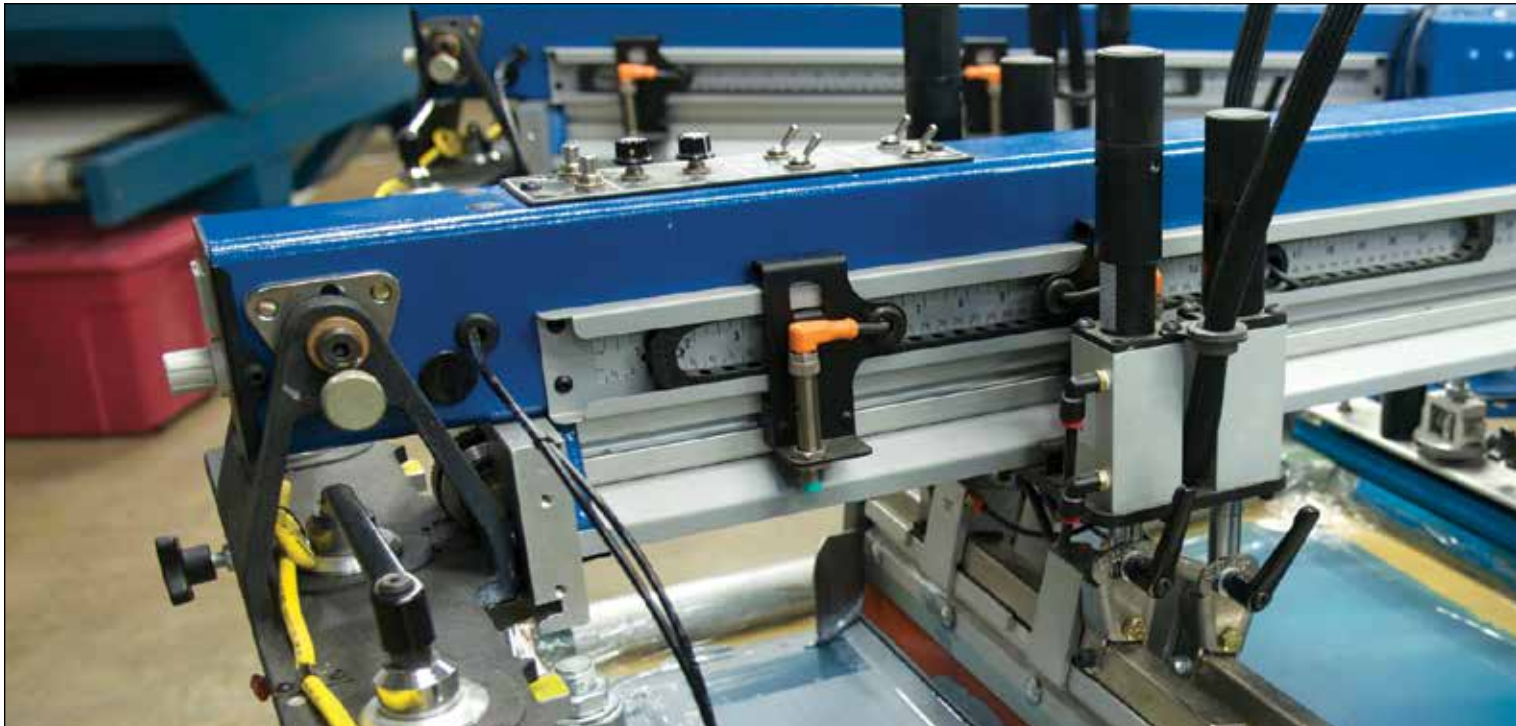
Nook/Thomson Modular Linear Actuators used in an automated silkscreen device.
