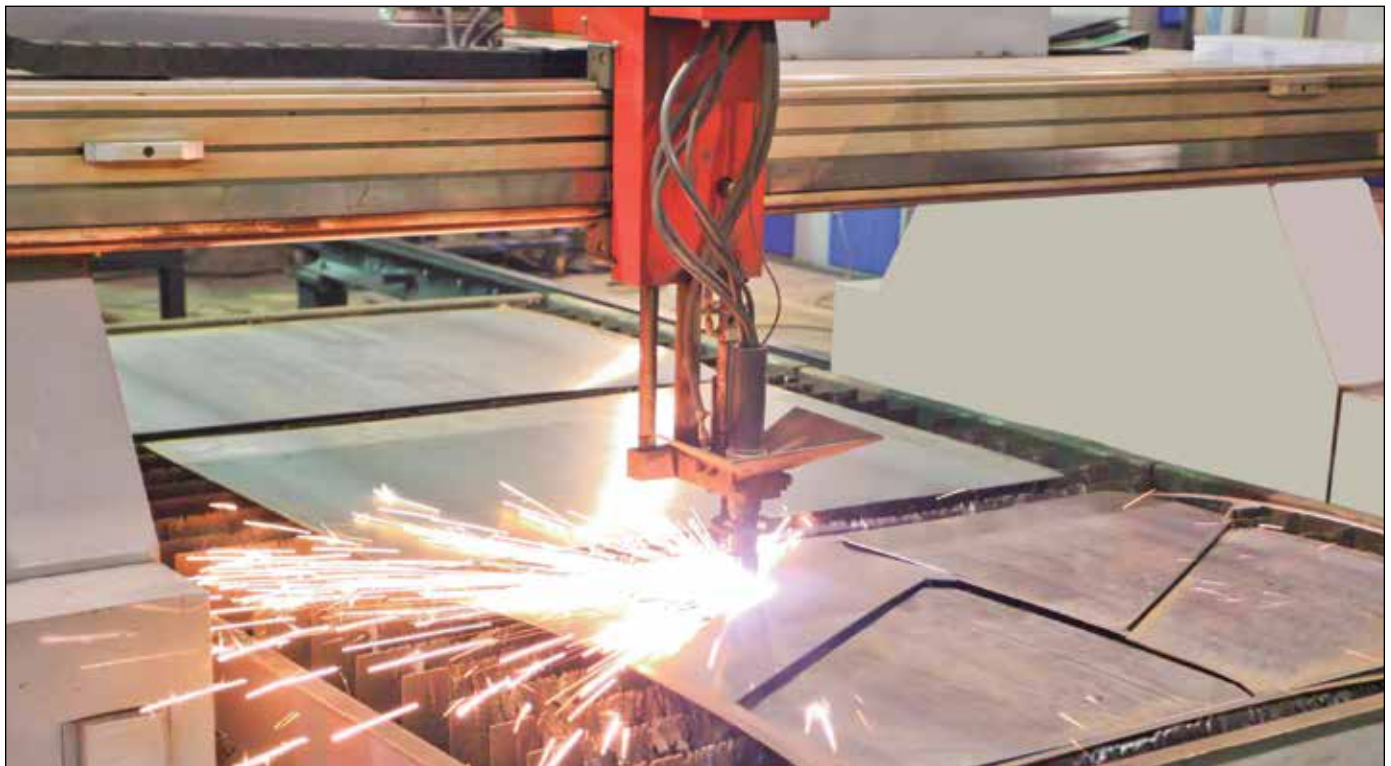
Nook/Thomson Modular Linear Actuators used in a plasma cutting application.
