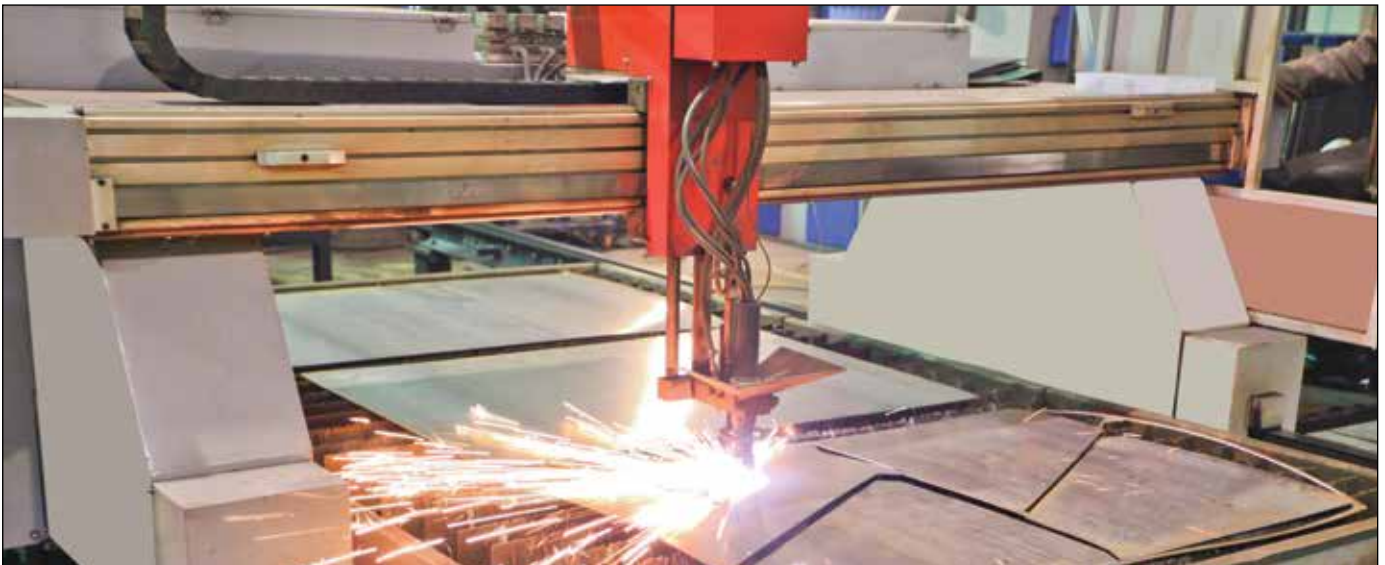
Nook/Thomson Modular Linear Actuators used in a plasma cutting application.
