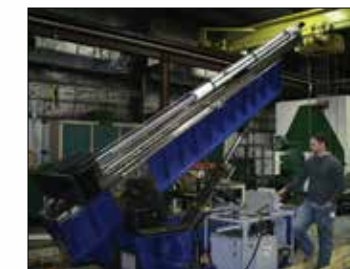
Convertible Test System 20,000 lb load - 100" CC
